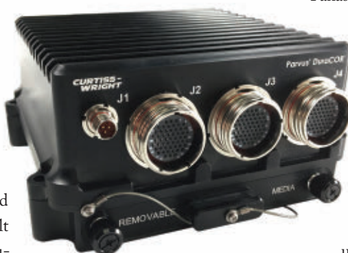
▲ The Parvus DuraCOR 313 from Curtiss-Wright is an ultra-small form factor (USFF) rugged embedded computer based on a low-power, quad-core Intel Atom x6400E Series (Elkhart Lake) processor equipped with modularity for add-on I/O cards and data storage in a fanless IP67-rated miniature design.
