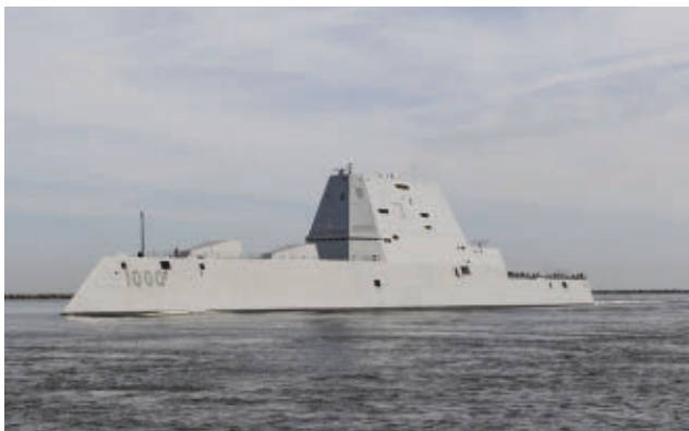
▲ The U.S. Navy's three Zumwalt-class (DDG 1000) destroyers are powered by an intermediate type integrated power system — perennial goal for the surface fleet.
